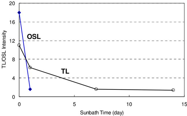
Fig. 4. Sunbath test for TL and OSL samples
