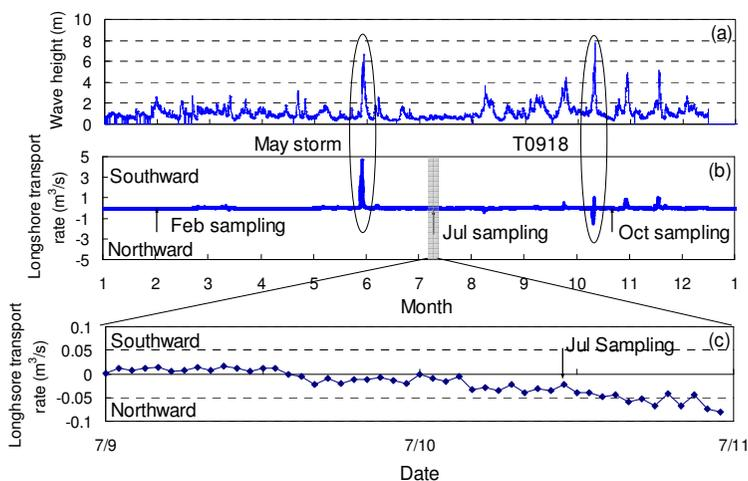
Fig. 3. Temporal variation of significant wave height and longshore sand transport rate estimated from the CERC formula along the Miyazaki Coast in 2009
