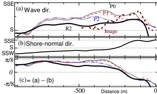
Fig. 11 Alongshore distributions of (a) wave directions, (b) shore-normal directions, and (c) difference between (a) and (b). Distance is from the east tip of the spit. (positive in eastward) P1, P2 and P3 denote the regular incident wave cases with  $Q=0, 140, \text{ and } 280\text{m}^3/\text{s}$ , respectively whereas R2 denotes the unidirectional random wave case with  $Q=280\text{m}^3/\text{s}$ .
