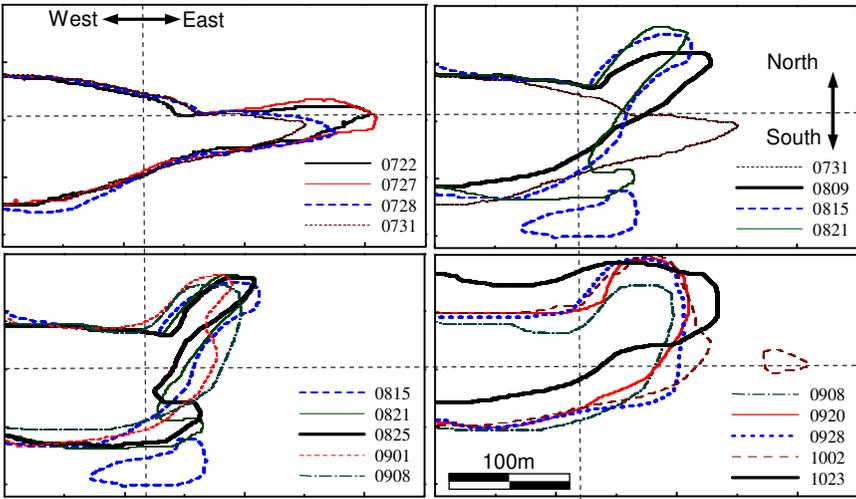
Fig.4 Time-varying profiles of the east tip of sand spit and Tenryu river and field survey setups
