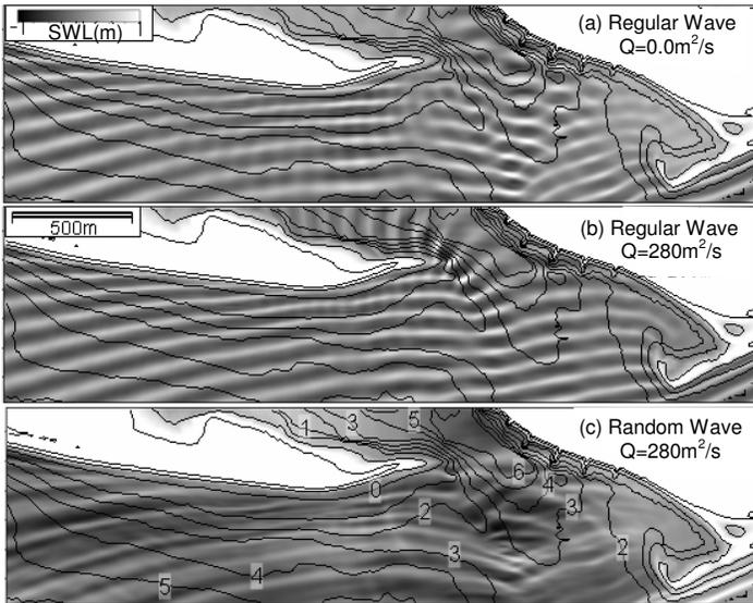
Fig. 10 Comparisons of predicted instantaneous surface water profiles.
