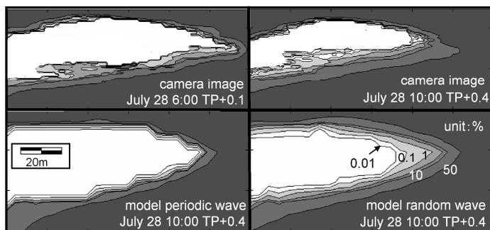
Fig. 9 Horizontal distributions of observed (top two) and predicted (bottom two) inundation rates.
