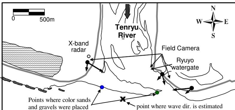
Fig.1 Plane view of the Tenryu river and field survey setups
