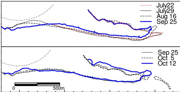
Fig.2 Spatial profiles of the sand spit at different time measured by GPS.
