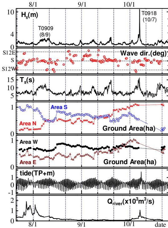
Fig.5 Time-series of various hydrodynamics and ground area in north, south, east and west area.
